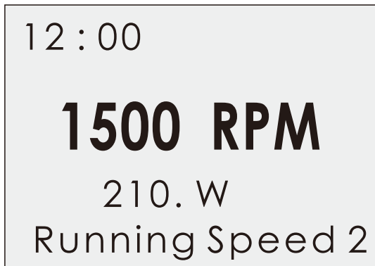
Normal Operating Interface Display 正常运转界面显示
